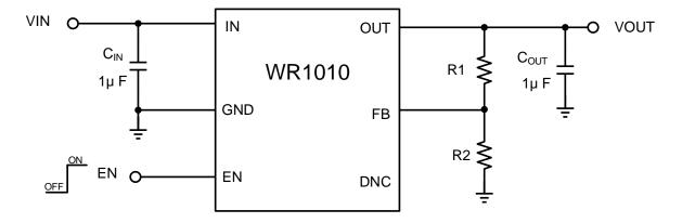
$$V_{OUT} = V_{FB} \times \left(1 + \frac{R_1}{R_2}\right)$$
